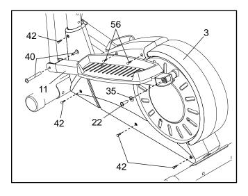
Remove the Pedal Arm Bolt Set (40), the M10 x 25mm Patch Screw (22), and the M10 Washer (35) from the Left Pedal Arm (11). Remove the Left Pedal Arm. Next, remove the two M4 x 25mm Screws (56) and the four M4 x 16mm Screws (42) from the Left Side Shield (3).
